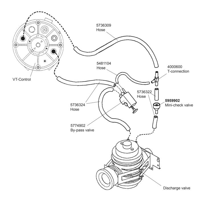
VT-Control and Discharge valve do not include in (P/N 5774903)
