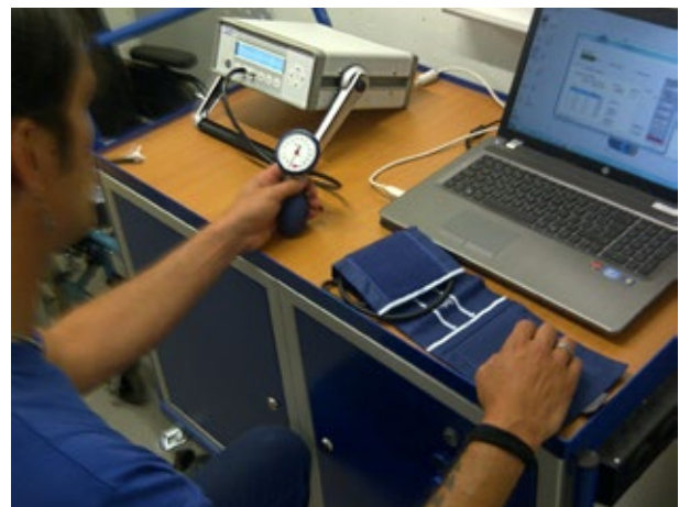
In practice: Blood pressure monitors in the nursing home Solina in Spiez (Switzerland) are calibrated by the technician responsible.
